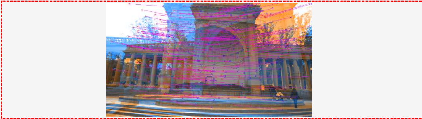
Figure 3: Detection and Matching of Feature Points pairwise. From Temple dataset ( Knapitsch et al. 2017 ).
